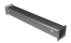
Hammond 1487SS series pull-through wireway, 4 x 4 x 36in, 304 stainless steel, #4 brush finish, screw clamps, NEMA 4/4X/12.
