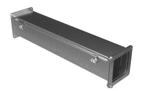
Hammond 1487SS series pull-through wireway, 4 x 4 x 24in, 304 stainless steel, #4 brush finish, screw clamps, NEMA 4/4X/12.
