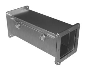
Hammond 1487SS series pull-through wireway, 4 x 4 x 12in, 304 stainless steel, #4 brush finish, screw clamps, NEMA 4/4X/12.
