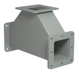
Hammond 1487 series pull-through wireway fitting, tee, 2.5 x 2.5in, carbon steel, ANSI 61 gray, powder coat finish, NEMA 12. For use with 1487 series wireway.
