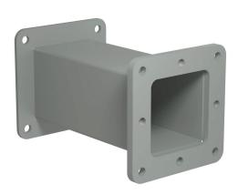
Hammond 1487 series pull-through wireway fitting, nipple,  $2.5 \times 2.5 \times 6$  in, carbon steel, ANSI 61 gray, powder coat finish, NEMA 12. For use with 1487 series wireway.
