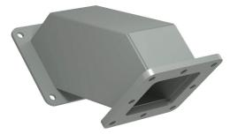
Hammond 1487 series pull-through wireway fitting, 90-degree elbow, 2.5 x 2.5in, carbon steel, ANSI 61 gray, powder coat finish, NEMA 12. For use with 1487 series wireway.
