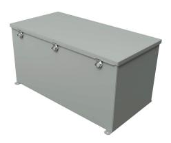
Hammond wiring trough, 12 x 12 x 24in (HxDxL), NEMA 1/4/12, carbon steel, ANSI 61 gray, powder coat finish, single-door.
