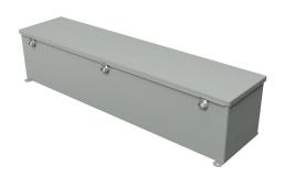
Hammond wiring trough, 8 x 8 x 36in (HxDxL), NEMA 1/4/12, carbon steel, ANSI 61 gray, powder coat finish, single-door.
