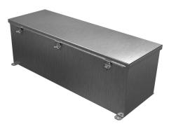
Hammond wiring trough,  $8 \times 8 \times 24$ in (HxDxL), NEMA 1/4/4X/12, 304 stainless steel, #4 brush finish, single-door.
