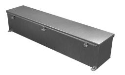
Hammond wiring trough, 6 x 6 x 30in (HxDxL), NEMA 1/4/4X/12, 304 stainless steel, #4 brush finish, single-door.
