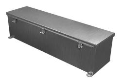
Hammond wiring trough,  $6 \times 6 \times 24$ in (HxDxL), NEMA 1/4/4X/12, 304 stainless steel, #4 brush finish, single-door.
