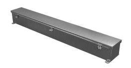
Hammond wiring trough, 4 x 4 x 36in (HxDxL), NEMA 1/4/4X/12, 304 stainless steel, #4 brush finish, single-door.
