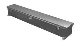
Hammond wiring trough,  $4 \times 4 \times 30$  in (HxDxL), NEMA 1/4/4X/12, 304 stainless steel, #4 brush finish, single-door.
