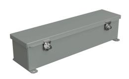
Hammond wiring trough, 4 x 4 x 18in (HxDxL), NEMA 1/4/12, carbon steel, ANSI 61 gray, powder coat finish, single-door.
