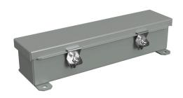
Hammond wiring trough,  $2.5 \times 2.5 \times 12$ in (HxDxL), NEMA 1/4/12, carbon steel, ANSI 61 gray, powder coat finish, single-door.
