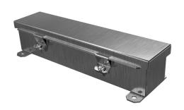
Hammond wiring trough,  $2.5 \times 2.5 \times 12$ in (HxDxL), NEMA 1/4/4X/12, 304 stainless steel, #4 brush finish, single-door.
