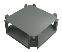
Hammond lay-in wireway fitting, cross fitting,  $12 \times 6in$ , carbon steel, ANSI 61 gray, powder coat finish, quick-release clamps, NEMA 12. For use with 1485 series wireway.
