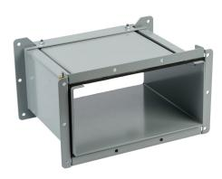
Hammond lay-in wireway fitting, adjustable fitting,  $12 \times 6 \times 2$  to 7in, carbon steel, ANSI 61 gray, NEMA 12.
