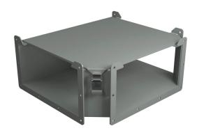
Hammond lay-in wireway fitting, tee, 12 x 6in, top opening, carbon steel, ANSI 61 gray, powder coat finish, quick-release clamps, NEMA 12. For use with 1485 series wireway.
