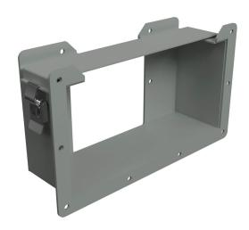
Hammond lay-in wireway fitting, reducer, 12 x 6in to 6 x 6in, edge-aligned opening, carbon steel, ANSI 61 gray, powder coat finish, quick-release clamps, NEMA 12. For use with 1485 series wireway.
