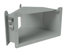
Hammond lay-in wireway fitting, 45-degree elbow, 12 x 6in, top opening, carbon steel, ANSI 61 gray, powder coat finish, quick-release clamps, NEMA 12. For use with 1485 series wireway.
