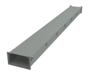
Hammond 1485 series lay-in wireway,  $12 \times 6 \times 120$ in, carbon steel, ANSI 61 gray, powder coat finish, quick-release clamps, NEMA 12.
