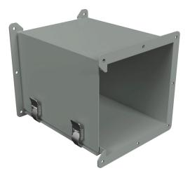
Hammond lay-in wireway fitting, clockwise transposition, 8 x 8in, carbon steel, ANSI 61 gray, powder coat finish, quick-release clamps, NEMA 12. For use with 1485 series wireway.
