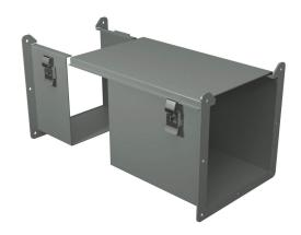
Hammond lay-in wireway fitting, cut-off fitting, 8 x 8 x 9 to 15in, carbon steel, ANSI 61 gray, powder coat finish, quick-release clamps, NEMA 12. For use with 1485 series wireway.
