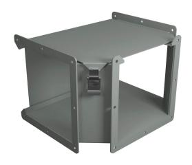
Hammond lay-in wireway fitting, tee, 8 x 8in, outside opening, carbon steel, ANSI 61 gray, powder coat finish, quick-release clamps, NEMA 12. For use with 1485 series wireway.
