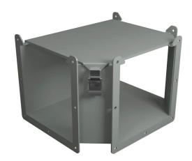
Hammond lay-in wireway fitting, tee, 8 x 8in, top opening, carbon steel, ANSI 61 gray, powder coat finish, quick-release clamps, NEMA 12. For use with 1485 series wireway.
