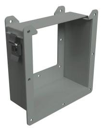
Hammond lay-in wireway fitting, reducer, 8 x 8in to 6 x 6in, edgealigned opening, carbon steel, ANSI 61 gray, powder coat finish, quick-release clamps, NEMA 12. For use with 1485 series wireway.
