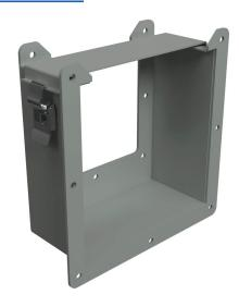
Hammond lay-in wireway fitting, reducer,  $8 \times 8$  in to  $6 \times 6$  in, edgealigned opening, carbon steel, ANSI 61 gray, quick-release clamps, NEMA 12.
