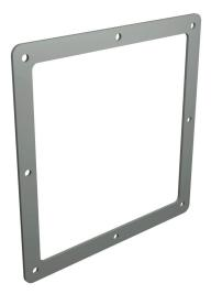
Hammond wireway fitting, box connector, 8 x 8in, carbon steel, ANSI 61 gray, powder coat finish, NEMA 12. For use with 1485 series wireway.
