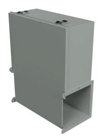
Hammond lay-in wireway fitting, junction box, 18 x 21.87 x 8in, carbon steel, ANSI 61 gray, powder coat finish, quick-release clamps, NEMA 12. For use with 1485 series wireway.
