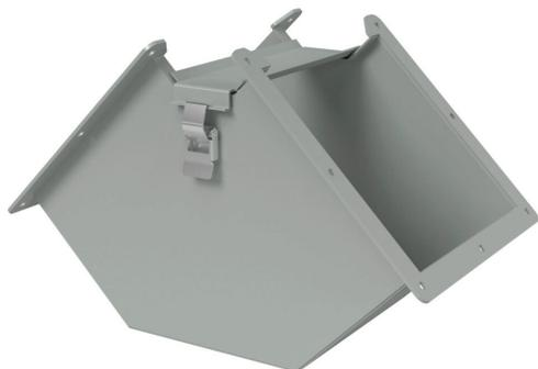
Hammond lay-in wireway fitting, 90-degree elbow, 8 x 8in, inside opening, carbon steel, ANSI 61 gray, powder coat finish, quick-release clamps, NEMA 12. For use with 1485 series wireway.
