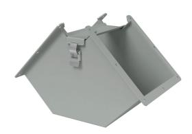
Hammond lay-in wireway fitting, 90-degree elbow, 8 x 8in, inside opening, carbon steel, ANSI 61 gray, powder coat finish, quick-release clamps, NEMA 12. For use with 1485 series wireway.
