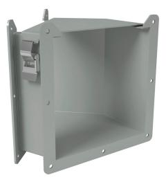
Hammond lay-in wireway fitting, 45-degree elbow, 8 x 8in, top opening, carbon steel, ANSI 61 gray, powder coat finish, quick-release clamps, NEMA 12. For use with 1485 series wireway.
