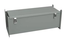
Hammond lay-in wireway,  $8 \times 8 \times 24$ in, carbon steel, ANSI 61 gray, quick-release clamps, NEMA 12.
