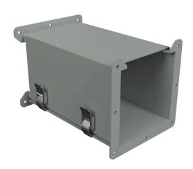
Hammond lay-in wireway fitting, counter-clockwise transposition, 6 x 6in, carbon steel, ANSI 61 gray, powder coat finish, quick-release clamps, NEMA 12. For use with 1485 series wireway.
