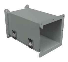
Hammond lay-in wireway fitting, clockwise transposition, 6 x 6in, carbon steel, ANSI 61 gray, powder coat finish, quick-release clamps, NEMA 12. For use with 1485 series wireway.
