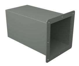
Hammond pull-through wireway fitting, cut-off fitting, 6 x 6 x up to 12in, carbon steel, ANSI 61 gray, powder coat finish, NEMA 12. For use with 1485 series wireway.
