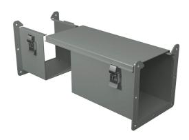
Hammond lay-in wireway fitting, cut-off fitting, 6 x 6 x 9 to 15in, carbon steel, ANSI 61 gray, powder coat finish, quick-release clamps, NEMA 12. For use with 1485 series wireway.
