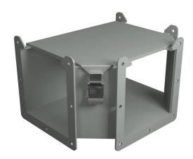
Hammond lay-in wireway fitting, tee, 6 x 6in, top opening, carbon steel, ANSI 61 gray, powder coat finish, quick-release clamps, NEMA 12. For use with 1485 series wireway.
