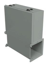
Hammond lay-in wireway fitting, junction box, 16 x 17.87 x 6in, carbon steel, ANSI 61 gray, powder coat finish, quick-release clamps, NEMA 12. For use with 1485 series wireway.
