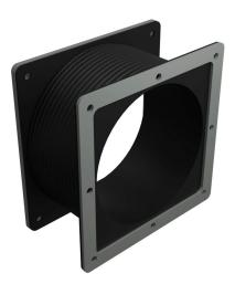
Hammond pull-through wireway fitting, flexible fitting, 6 x 6 x 3 to 10in, GortiflexTM bellows with carbon steel flanges, ANSI 61 gray, powder coat finish, NEMA 12. For use with 1485 and 1487 series wireway.
