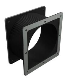
Hammond pull-through wireway fitting, flexible fitting, 6 x 6 x 3 to 10in, GortiflexTM bellows with carbon steel flanges, ANSI 61 gray, NEMA 12.
