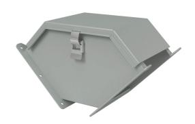
Hammond lay-in wireway fitting, 90-degree elbow, 6 x 6in, outside opening, carbon steel, ANSI 61 gray, powder coat finish, quick-release clamps, NEMA 12. For use with 1485 series wireway.
