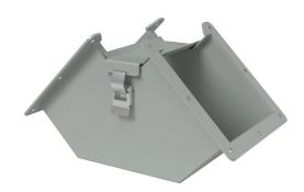
Hammond lay-in wireway fitting, 90-degree elbow, 6 x 6in, inside opening, carbon steel, ANSI 61 gray, powder coat finish, quick-release clamps, NEMA 12. For use with 1485 series wireway.
