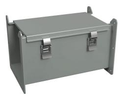
Hammond 1485 series lay-in wireway, 6 x 6 x 12in, carbon steel, ANSI 61 gray, powder coat finish, quick-release clamps, NEMA 12.
