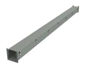
Hammond 1485 series lay-in wireway, 6 x 6 x 120in, carbon steel, ANSI 61 gray, powder coat finish, quick-release clamps, NEMA 12.
