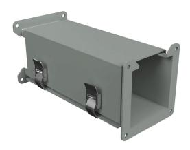
Hammond lay-in wireway fitting, counter-clockwise transposition, 4 x 4in, carbon steel, ANSI 61 gray, powder coat finish, quick-release clamps, NEMA 12. For use with 1485 series wireway.
