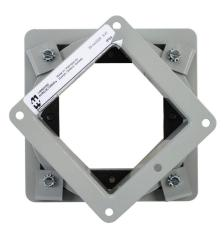
Hammond pull-through wireway fitting, standard swivel nipple, 4 x 4 x 2.25in, carbon steel, ANSI 61 gray, powder coat finish, NEMA 12. For use with 1485 series wireway.
