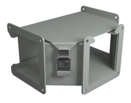
Hammond lay-in wireway fitting, tee, 4 x 4in, outside opening, carbon steel, ANSI 61 gray, powder coat finish, quick-release clamps, NEMA 12. For use with 1485 series wireway.
