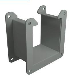
Hammond lay-in wireway fitting, nipple, 4 x 4 x 3in, carbon steel, ANSI 61 gray, powder coat finish, NEMA 12. For use with 1485 series wireway.
