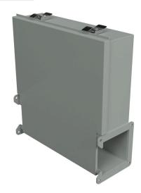
Hammond lay-in wireway fitting, junction box,  $14 \times 13.87 \times 4$ in, carbon steel, ANSI 61 gray, quick-release clamps, NEMA 12. For use with  $4 \times 4$ in wireway.
