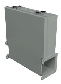
Hammond lay-in wireway fitting, junction box,  $14 \times 13.87 \times 4$ in, carbon steel, ANSI 61 gray, powder coat finish, quick-release clamps, NEMA 12. For use with 1485 series wireway.
