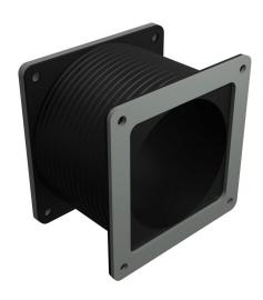
Hammond pull-through wireway fitting, flexible fitting,  $4 \times 4 \times 3$  to 10in, GortiflexTM bellows with carbon steel flanges, ANSI 61 gray, powder coat finish, NEMA 12. For use with 1485 and 1487 series wireway.
