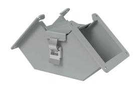
Hammond lay-in wireway fitting, 90-degree elbow, 4 x 4in, inside opening, carbon steel, ANSI 61 gray, powder coat finish, quick-release clamps, NEMA 12. For use with 1485 series wireway.
